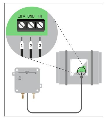
Fig. 2: Electrical connection of the device
