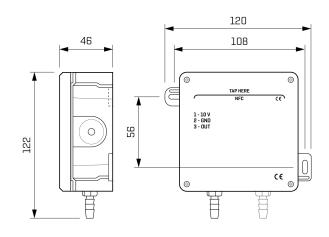
Fig. 1: Dimensions of the device without the cable in mm
